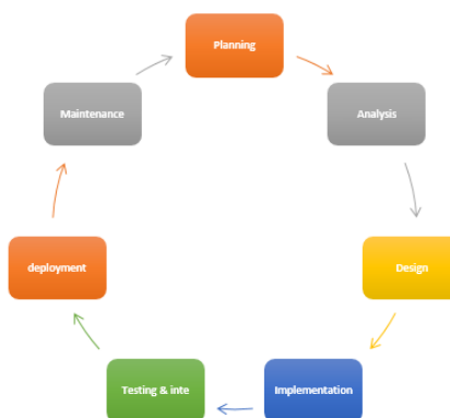
Figure 1. Stages of the System Development Life Cycle
